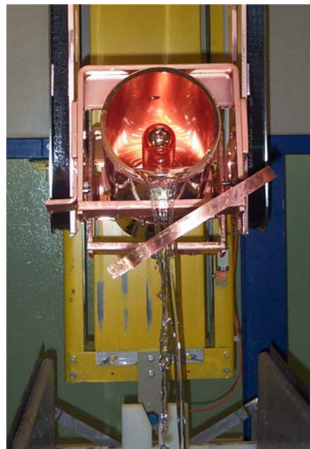
Fig. 1 – Shows an example of surface electrochemical polishing for particle accelerator application
