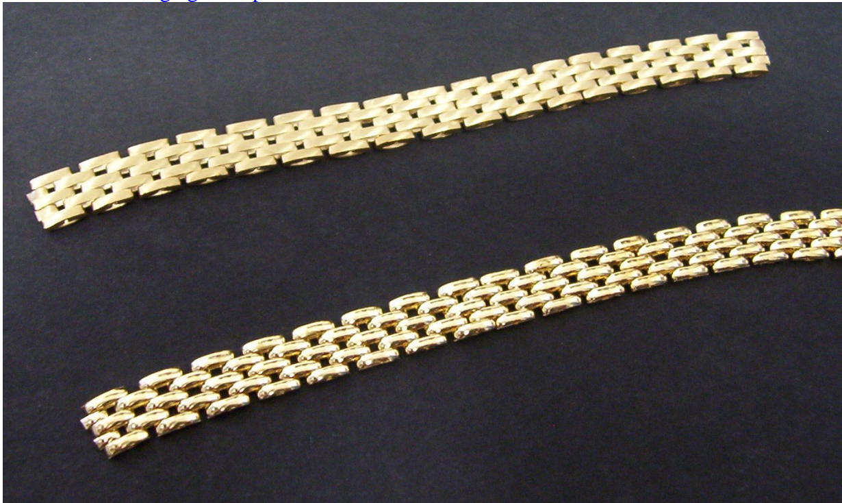
Fig. 5 - 18 carat golden chain before and after the electropolishing proposed by LNL.
