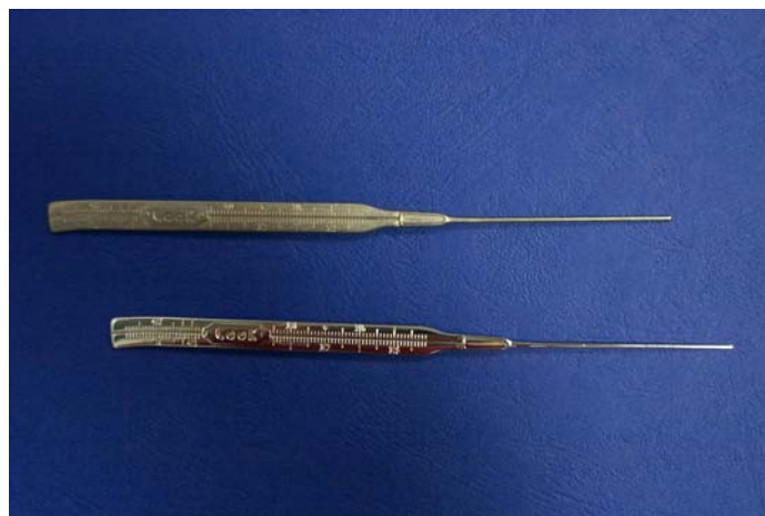
Fig. 4 - Glasses' stem before and after the electrolyte treatment.
